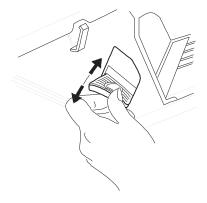
5 Firmly pull the tab and sealing tape straight out until all 22 inches (56 cm) of clear tape are completely out of the cartridge.
